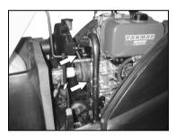
Check round belts and V-belts for tightness, wear and damage
