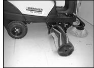
> Push main brush into main brush box and position it onto the driving peg
