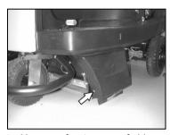
Unscrew front screw of side panelling
