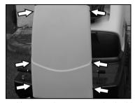
Unscrew the screws at both sides of the covering
