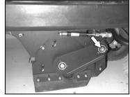
> Screw out screw at main brush bracket
