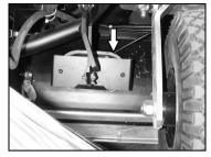
Vacuum canister for lowering the side brush (to the left and next to the front wheel viewed from the front
