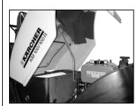
In its open position the unit cover is secured by a stay bar.
