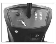
Elapsed-time meter indicates maintenance interval times.
