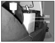
The oil level must be between the "MIN" and "MAX" marks.
