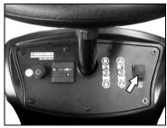
> Press filter cleaning switch briefly. The dust filter is cleaned for approx. 15 seconds. Do not open the unit cover during this period.
