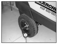
> The air pressure in the rear tyres must be set to 6 bar.
