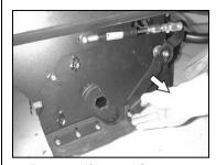
> Remove lifting rod from peg
